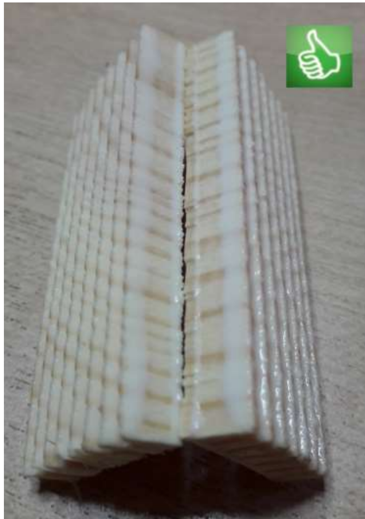
Picture 3: Example of approved adhesive application.
