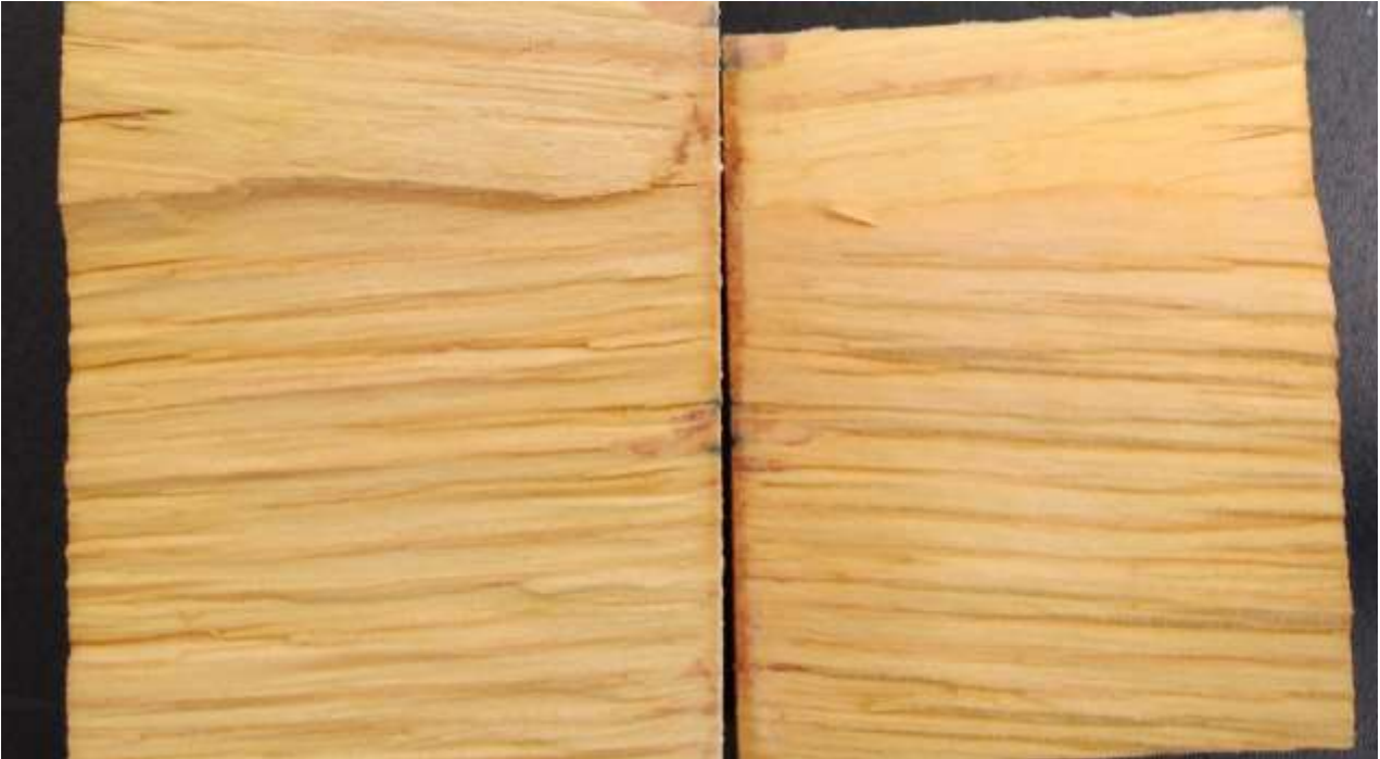
Picture 2: Surface after splitting and treated with iodine. Wood failure
