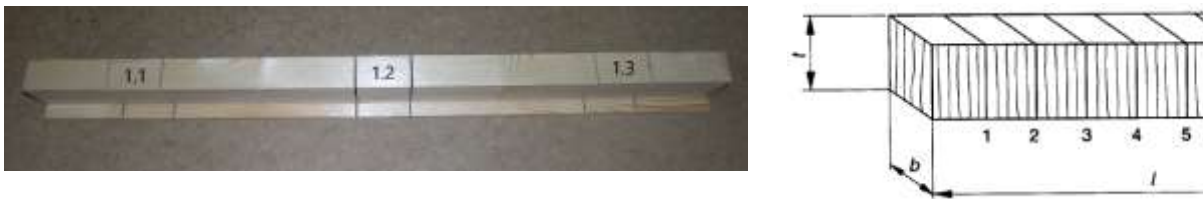
Figure 11. Positions of samples from a blank. Each blank is about 1 m long.
