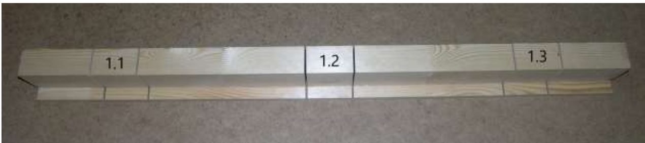
Figure 9. Positions of samples from a blank. Each blank is about 1 m long.
