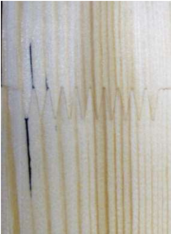
Picture 1: Cracks formed from finger bottoms - not accepted
