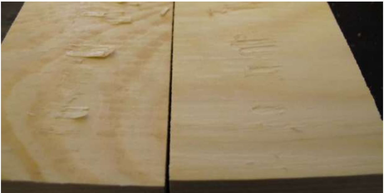
Picture 4: Surface after splitting - adhesive failure
