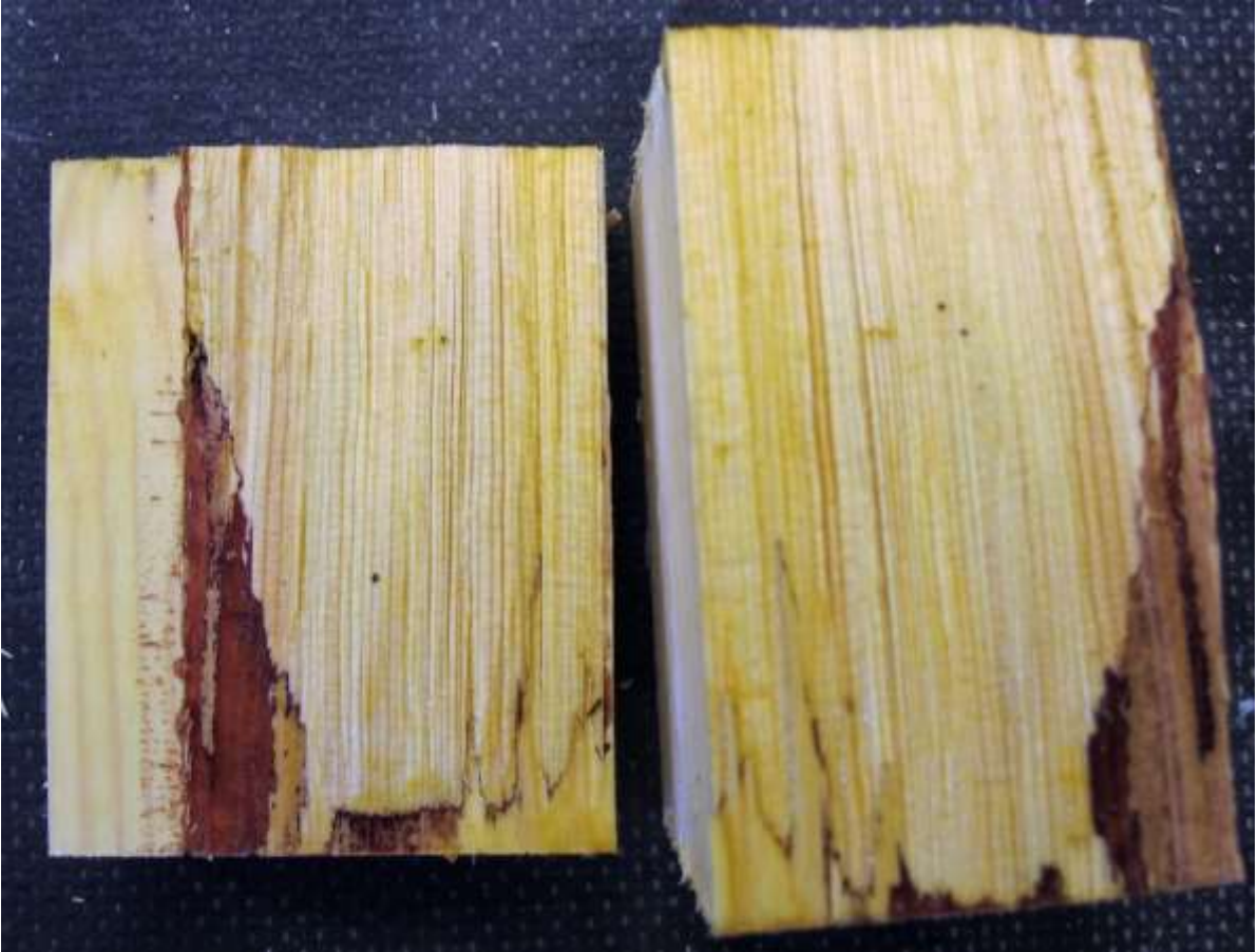
Picture 4: Surface after splitting - adhesive failure
